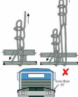
The greater the angle of the lashing to the load the greater the lashing tension will be. Angles less than 30° are not recommended.
