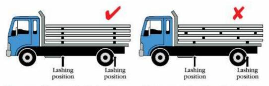
Dunnage needs to be vertically aligned to minimise movement when under lashings. The dunnage is placed irregularly and could loosen or overtighten lashings when the vehicle is operating.
